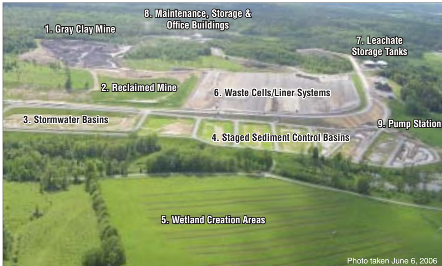
Aerial view designating various locations within the new landfill that will accept 300,000 tons of solid waste per year at the present rate. An average of 50 trucks per day will unload their collections at the facility.
